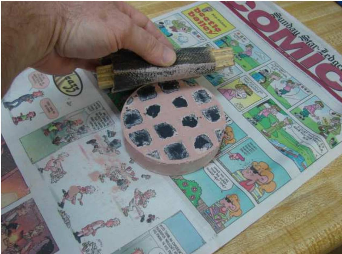
14. There may be a very thin film of plaster over some the tile faces, this will grind off in the first few grinding sessions. Let the tool dry/harden overnight.
