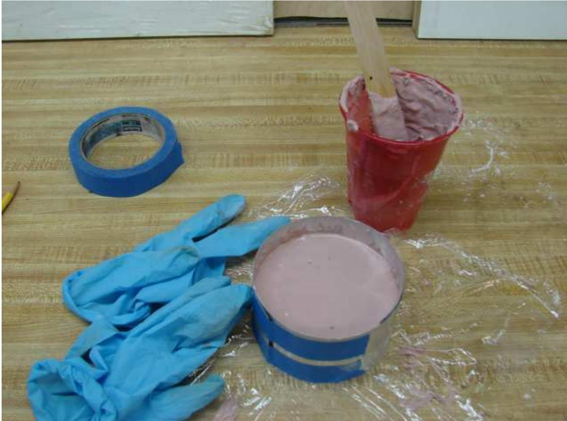
12. Remove the tape around the form allowing the form to unroll. Remove the form. The plaster is very weak at this point. Handle it with care.
