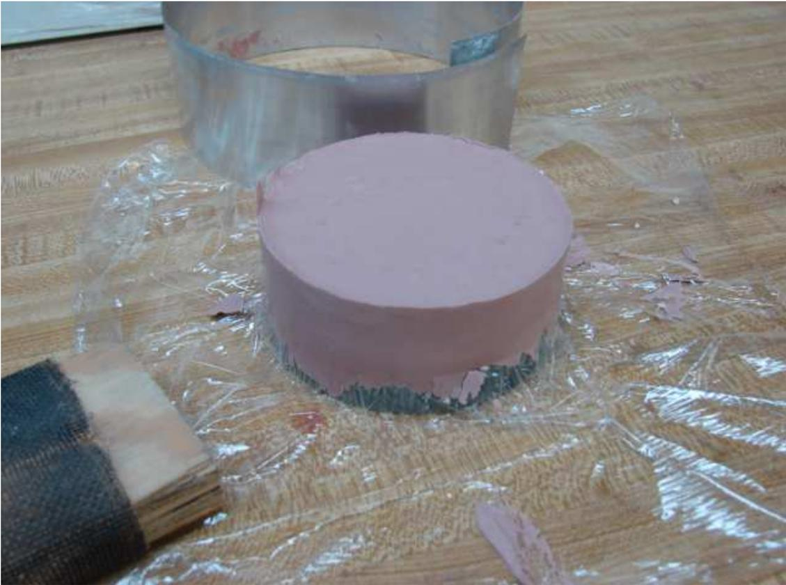
13. Smooth of the edges (gently) with an abrasive block. The plaster should be fairly soft. I used a wood block wrapped with some plastic door screening to wear away the soft plastic for this step.
