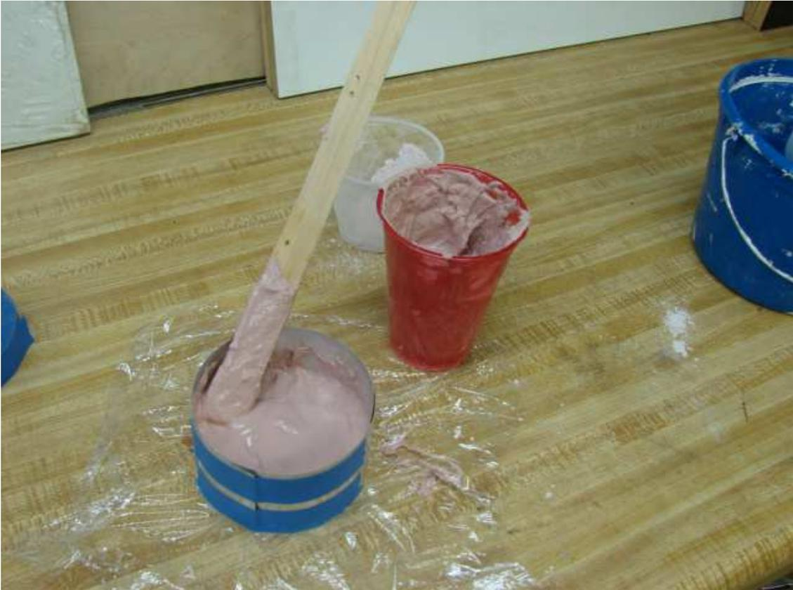
11. Pour more plaster to the desired thickness and smooth the top. Walk away for at least 20 minutes. Dental Plaster sets in less than 30 minutes. The surface of the plaster will begin to look dry and will be hard to the touch.
