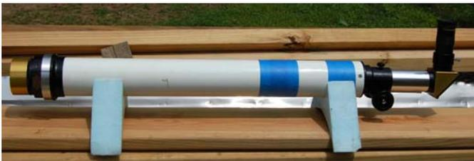
Coronado SolarMax Hydrogen-alpha filter and T-Max tuner adapted to a 60mm refractor.
