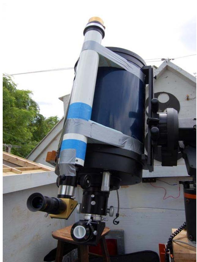
Solar 'Scope strapped to Clif's 10-inch Meade Schmidt-Cassegrain telescope. Note Coronado BF-10 blocking filter at the focuser.
